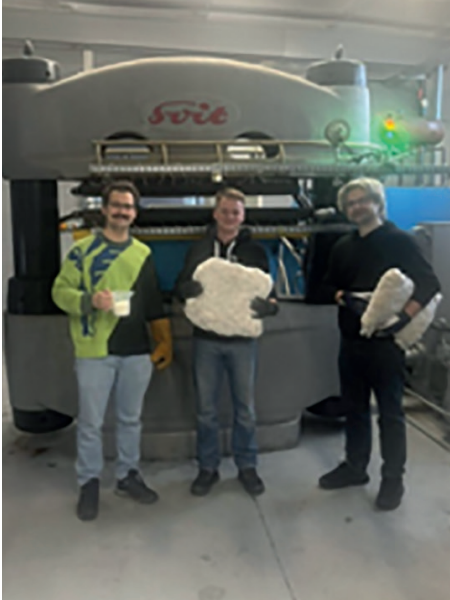
Pressing composite panels on a heated press.
