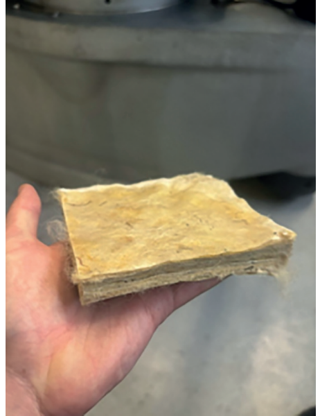
Compressed composite material based on sheep's wool and a biodegradable matrix.
