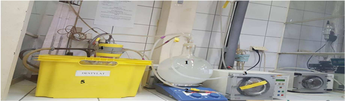
Photo 1. Testing installation for membrane distillation. 1. tank feed with immersed modules, 2. heating plate with mixing, 3. peristaltic pump, 4. distillate tank, 5. distillate tank with cooler. Own source.
